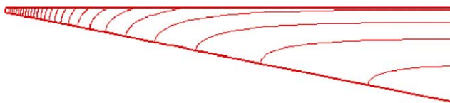
Fig. 2. Typical temperature structures at early stages of the flow development. Plotted here are the calculated temperature contours for Pr = 7 , Gr = 10^5 and A = 0.1 at the dimensionless time t = 0.02 . The dimensionless contour interval is 0.04.
